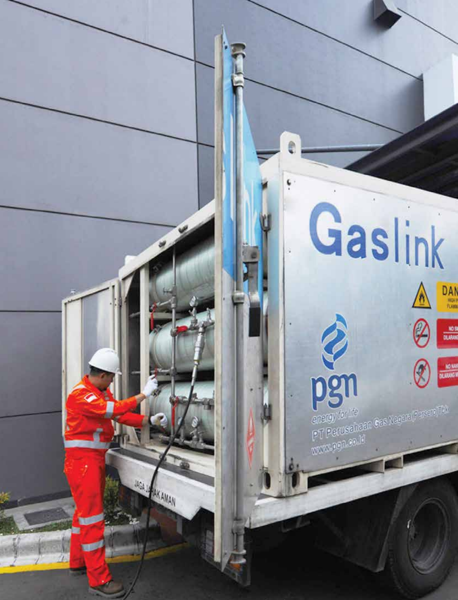
CNG Cradle (Gaslink), created by the PGASSOL Subsidiary for the support of the natural gas business in the commercial sector, especially for customers who have not crossed the gas pipeline. In addition, PGASSOL also performs maintenance and operation of CNG Cradle.
