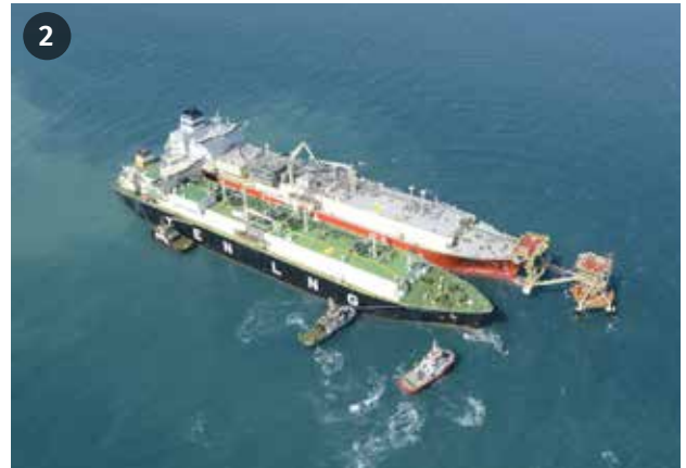
2. FSRU Lampung is unloading from LNG carrier vessel. In addition to having the ability to regasification, FSRU Lampung also has LNG gas storage.
